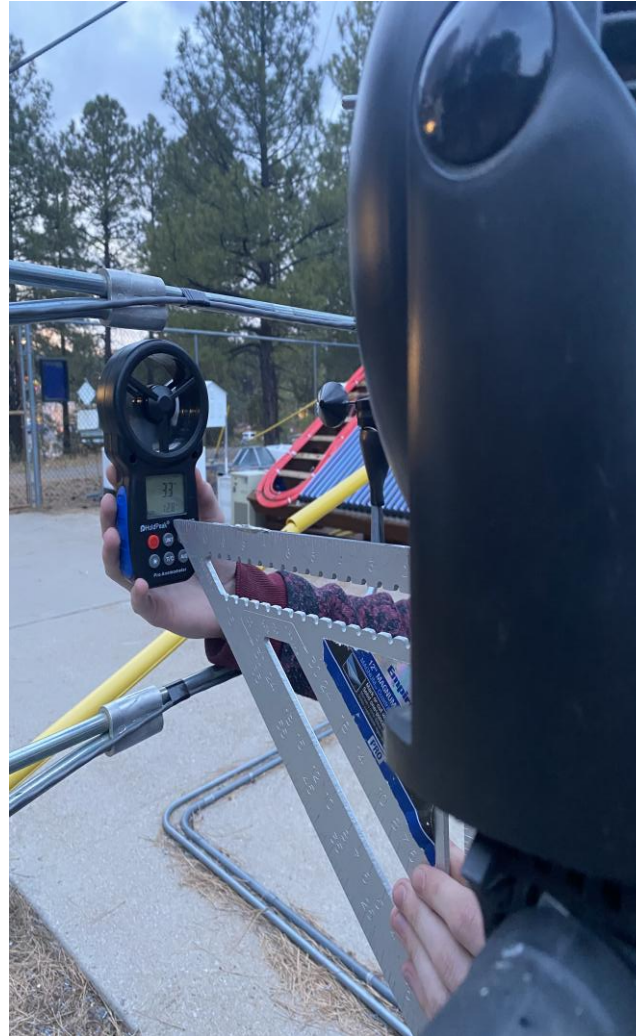
Figure 25: Handheld Anemometer Calibration Test
