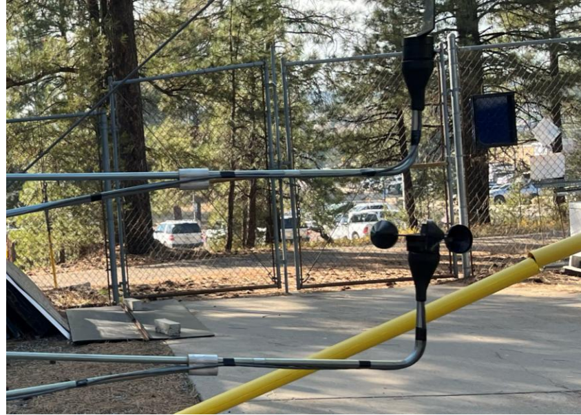
Figure 22: Wind Vane (top) and Anemometer (bottom)
