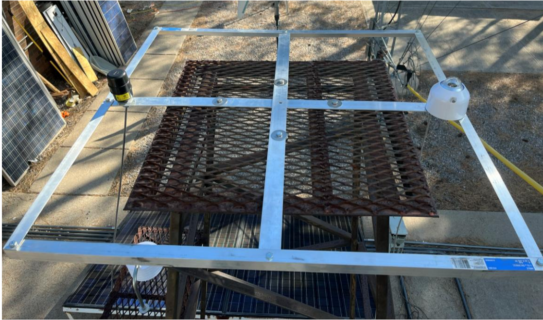
Figure 21: Barometric Pressure Sensor (left) and Pyranometer (right)
