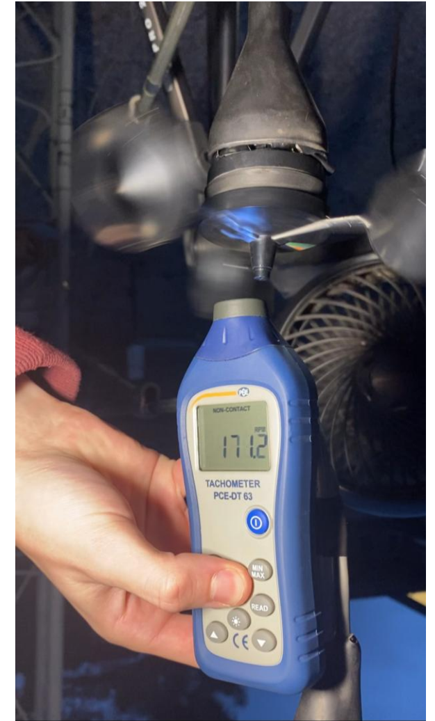
Figure 26: Rotation Speed Measurement Test
